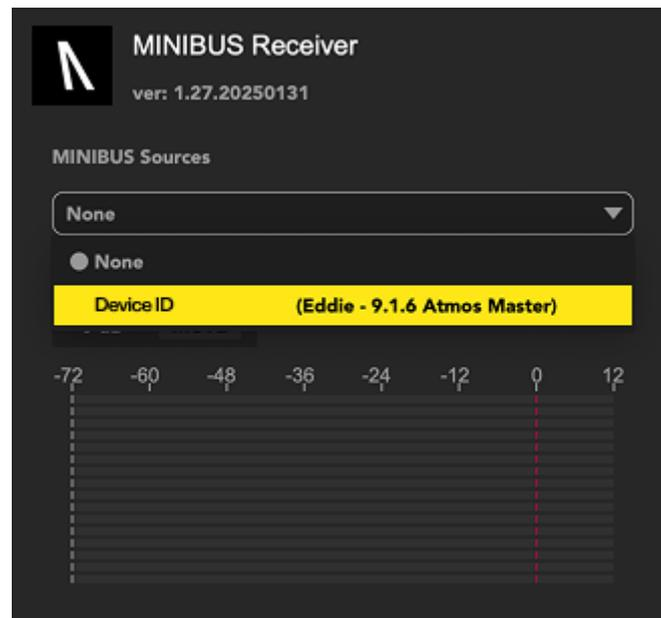
The MINIBUS Receiver scans your local network for available transmitters. Choose one of the transmitters from MINIBUS' drop down menu in order to receive a stream from it. The above image shows an incoming 9.1.6 NDI transmission from OMNIBUS 3.
