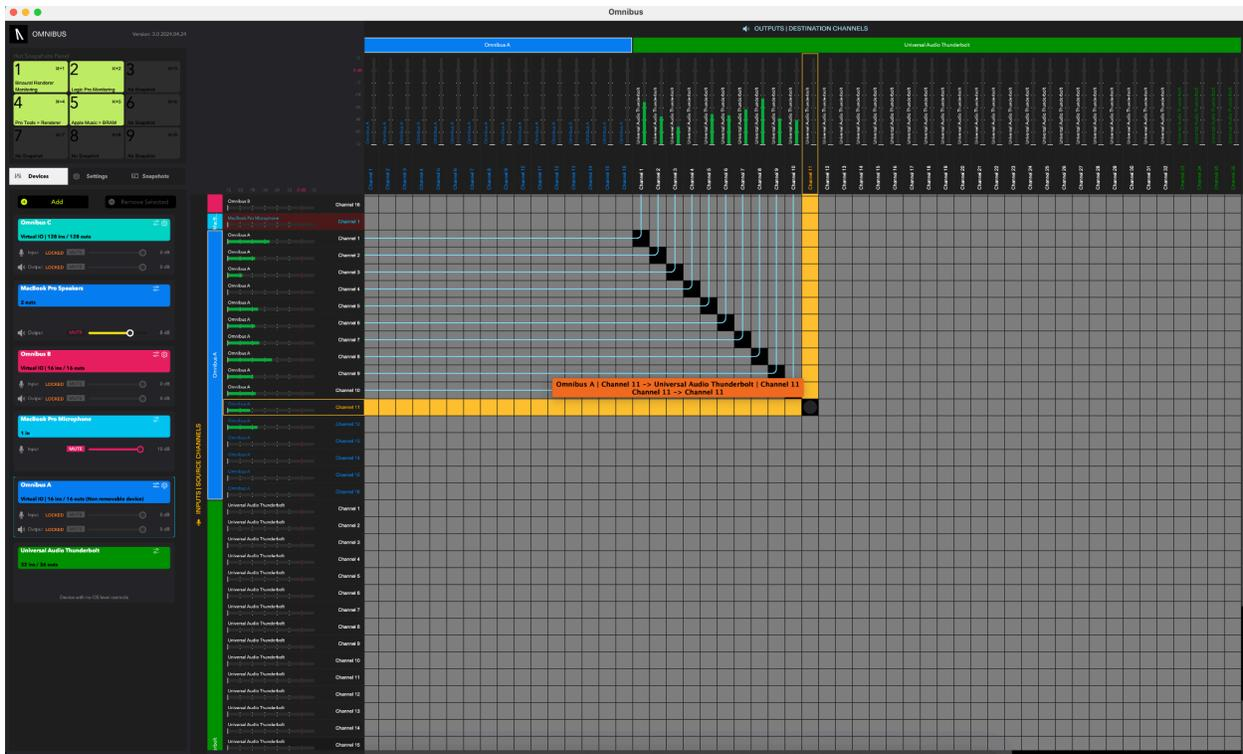
To route audio through the routing matrix, click on the corresponding cell to connect a source to a destination. For example, you can route the “MacBook built-in microphone” to channel 1 of OMNIBUS B.
