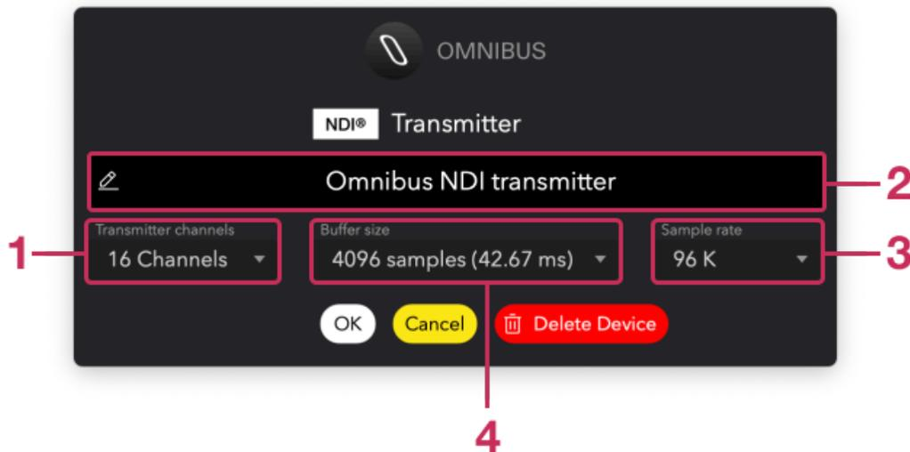
1. **I/O Channels:** Choose the channel count for your transmitter device, ranging from 2 to 128.
