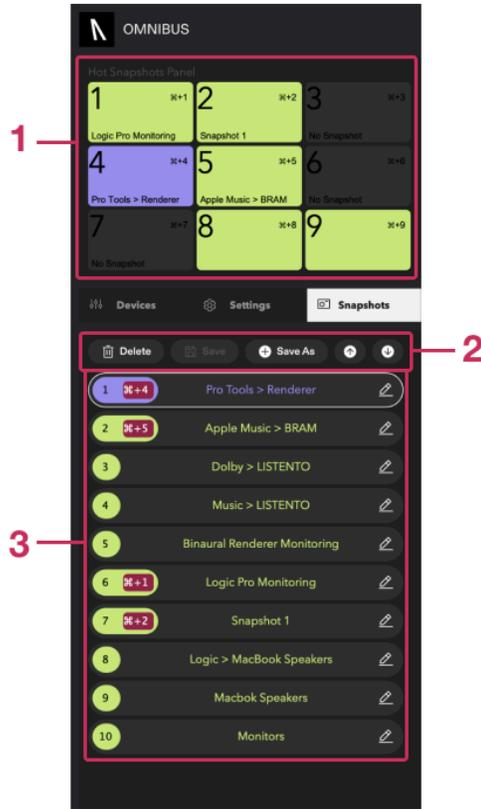
1. **Hot Snapshot Panel:** Users can assign up to nine snapshots in the Hot Snapshot Panel by right clicking on a snapshot. You can recall hot snapshots with key command Cmd + 1-9
